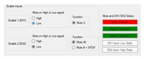
EN1 and EN2 inputs can be set to mute if the signal connected to these ports are logic high or logic low (24V or 0V). EN2 can also change function to either Mute All or to only Mute B + C (SPDIF).
