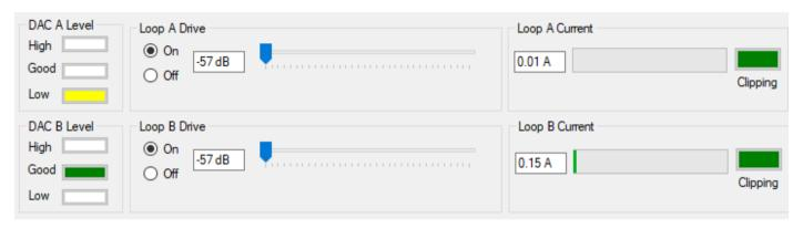
**DAC A/B Level** – Indicates the level of the audio signal being fed to each output channel's DAC. This is the signal level after pre-amp gain, processed by AGC, HPF, HFC, but before any Output drive level has been applied. Make sure to keep it in the "good" range.
