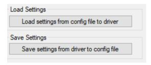
The software can save all settings stored on the driver to a config file. This can then be used to load these
