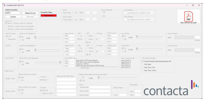
The only controls available at this point are "Refresh Port List" and "Connect". Select the COM port to which the VLD1 driver is connected and click "Connect" to make a connection attempt.
