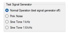
This feature provides the required signals needed for setting up a loop, negating the need for an external signal generator. Selecting any of these settings bypasses the signal from the audio inputs.
