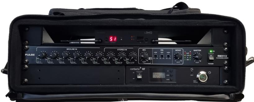
6. Switch on the Radio Frequency Transmitter, 12 Channel Microphone Mixer, and 1 Channel Microphone Receiver. Ensure the dials for Channel 1 and Channel 2 are set to Level 2.
