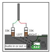
If connecting the unit to a 100V line, use two resistors with a voltage rating greater than 100V peak (200V peak-to-peak) as per the diagram on the left.
