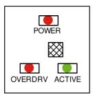
**POWER** - Constantly lit red to indicate the device is powered on. **ACTIVE** - Illuminates green when a loop is being driven correctly. **OVERDRIVE** - Becomes increasingly steady red as an audio signal increases. If it is continuously red, the drive level of the loop is too high and audio may be distorted.
