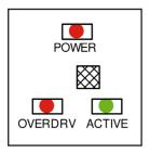
**POWER** - Constantly lit red to indicate the device is powered on. **ACTIVE** - Illuminates green when a loop is being driven correctly. **OVERDRIVE** - Becomes increasingly steady red as an audio signal increases. If it is continuously red, the drive level of the loop is too high and audio may be distorted.
